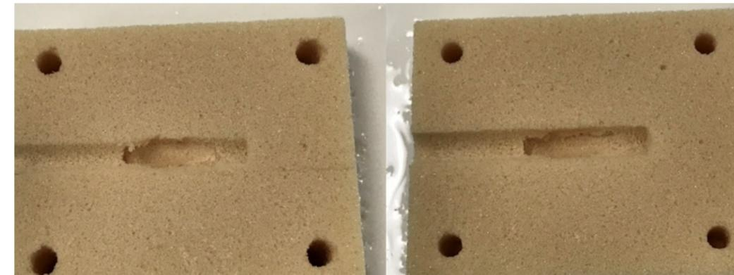
**Figure 7.** Photographs illustrating the subsidence pattern within the foam block from expansion of a SpineJack™ device.
