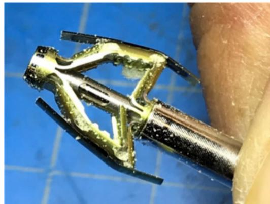
**Figure 9.** Photograph illustrating the SpineJack™ device after deployment in 10 pcf foam blocks. Note the asymmetrical and broken tine, indicating an inability to be fully deployed.
