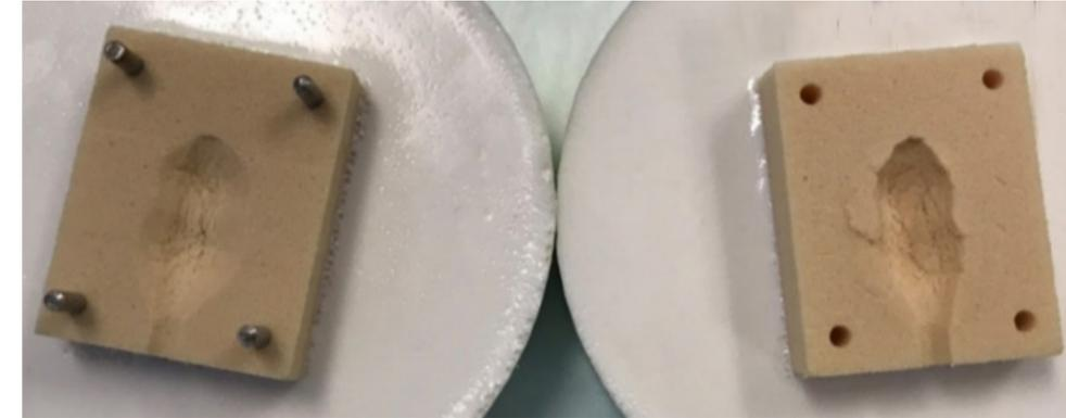
**Figure 6.** Photograph illustrating the subsidence pattern within the foam block from inflation of a Kyphon Xpander™ II IBT to a volume of 5.0 cc.
